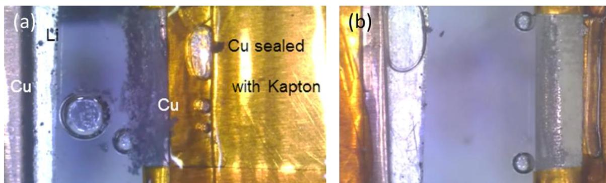
Figure 1. Operando microscopy observations of Li plating on (a) bare Cu and (b) polymer coated Cu current collectors.
